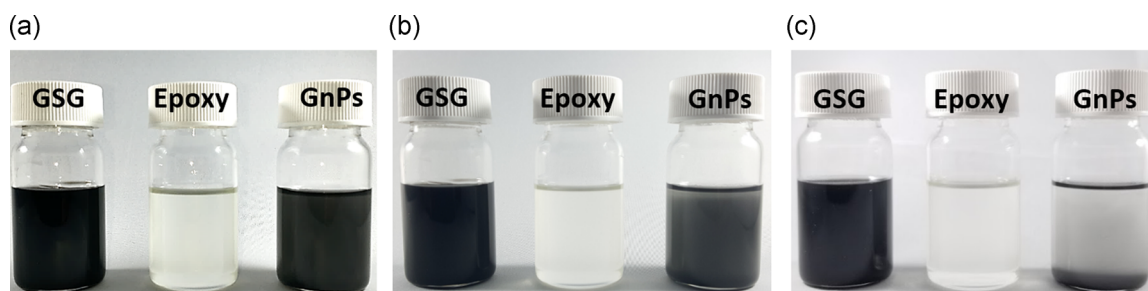
FIGURE 2 (a) Vials containing 0.1 wt% GSG in epoxy, pure epoxy, and 0.1 wt% GnPs in epoxy immediately after mixing, (b) after 1 week, and (c) after 1 year. The GSG remains dispersed in epoxy, while the GnPs in epoxy aggregate and result in a heterogeneous suspension. GnP, graphene nanoplatelet; GSG, gas-phase-synthesized graphene
