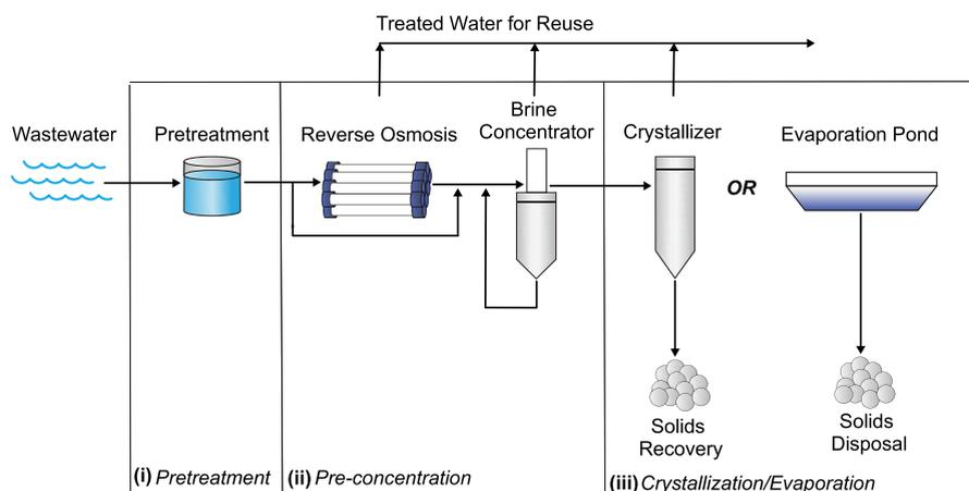
**Figure 3.** Conventional zero liquid discharge (ZLD) treatment scheme with (i) pretreatment, (ii) pre-concentration by reverse osmosis and/or a brine concentrator, and (iii) crystallization/evaporation by crystallizers and/or evaporation ponds. Figure adapted from Global Water Intelligence.<sup>93</sup>
