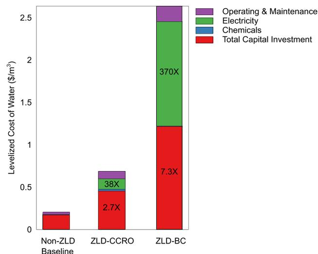
Figure 6. Levelized cost of water (LCOW) for the two ZLD scenarios (ZLD-CCRO and ZLD-BC) are compared with LCOW for the non-ZLD baseline scenario for Cherokee Generating Station. LCOW values are broken down into general cost categories. Further breakdown of the cost categories (i.e., detail of the  $\text{LCOW}_{\text{TCI}}$  and  $\text{LCOW}_{\text{elec}}$  values) is shown in Figure 7.
