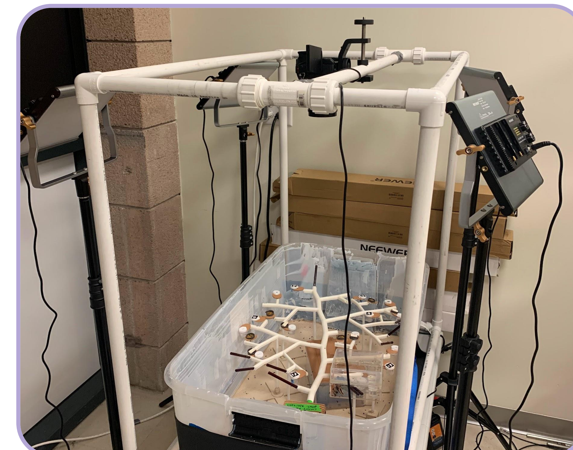
Fig. 2. Experimental Setup: The branch was placed into a bin, resting on slippery stands and a wooden block trunk. A camera and lights were set up for recording.
