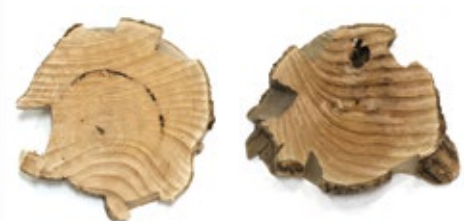
2 Detail of two cookies after waterjetting and CNC routing
