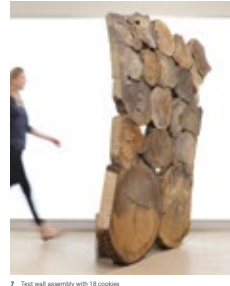
Test wall assembly with 18 cookies
