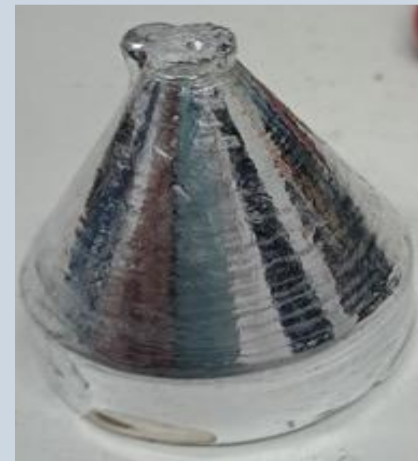
Tatur test for experimental shrinkage
