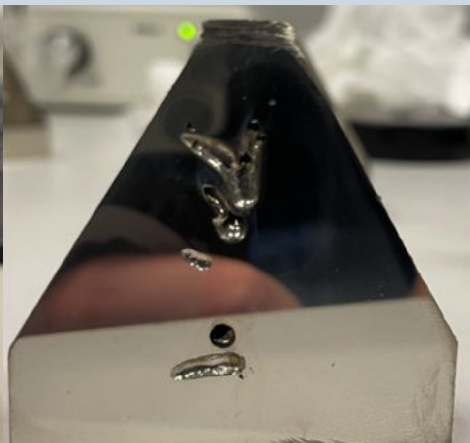
Low shrinkage (small cavity)
