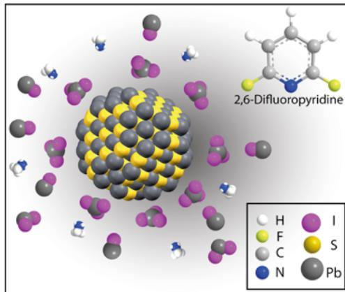
A schematic of a lead iodine/methyl ammonium lead iodide perovskite core/shell quantum dot suspended in 2,6-difluoropyridine, creating an ink that can be printed on surfaces to create photovoltaic cells. These quantum dots are roughly 3.2 nm in diameter.
