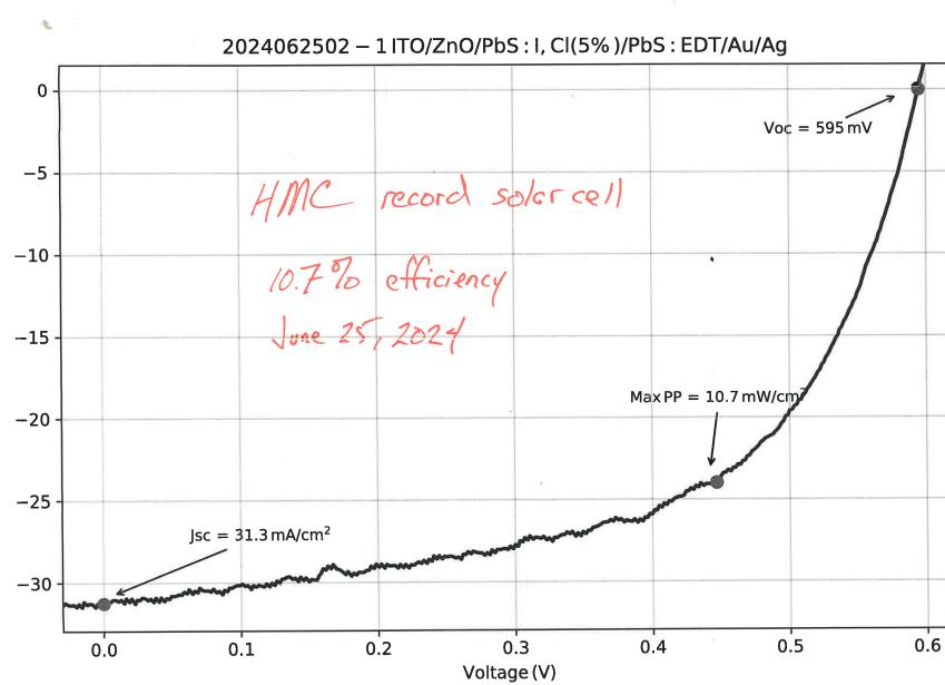
Current-voltage (power) curve showing current density (mA cm<sup>-2</sup>) as a function of applied voltage for a quantum dot solar cell employing lead sulfide quantum dots capped with lead iodide and lead chloride. The cell is 10.7% efficient in converting optical to electrical power.
